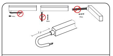
Do not pull the cable, otherwise it may disable the function of the connector and lead to water ingression. It's recommended to keep at least 60mm cable in the natural state at the cable joint with light.
